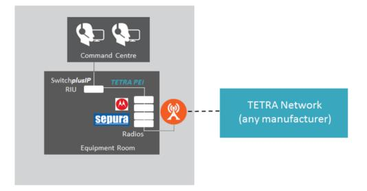
Support for **multiple TETRA networks** has been added to allow large organisations to centralise access and obtain seamless control of multiple independent TETRA networks. This functionality allows greater co-ordination and flexibility to control room operators; from the one console, operators can communicate with and patch together individual subscribers and talkgroups across the networks.
